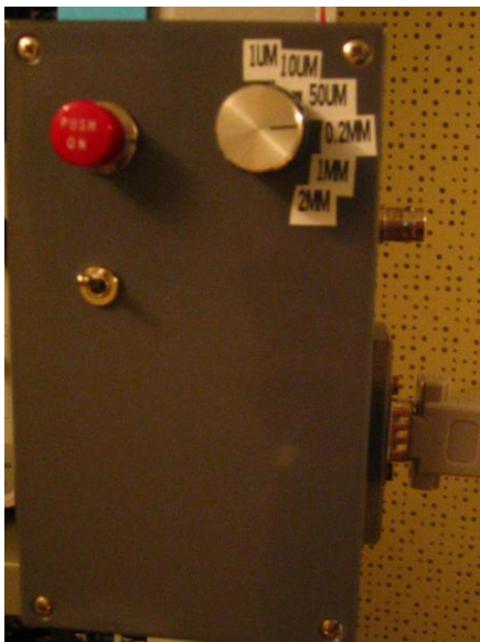
Figure 4 Finished Box for Piezo-motor M-674.164 control
