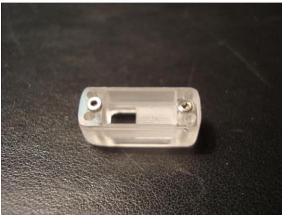
Figure 11 Finished Recording array chamber
