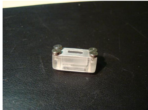
Figure 11 Finished Recording array chamber
