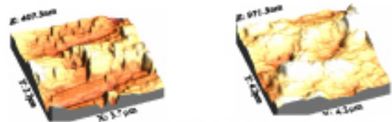
Fig. 7. AFM images of implant never put in place and one that has been incorporated in bone
